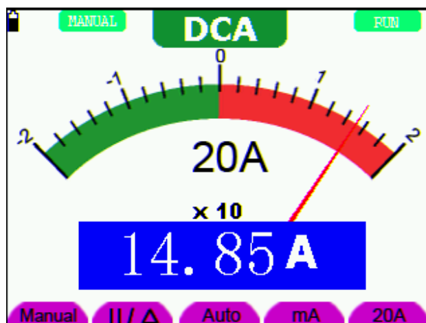
figure 25: DC Current Measurement for 20A
