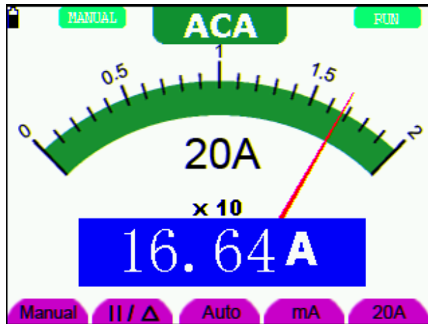
figure 27: AC Current Measurement for 20A
