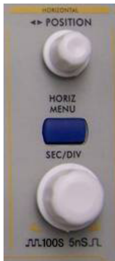
Fig. 9 Horizontal Control Zone
