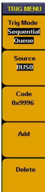
Fig. 82 Sequential queue trigger
