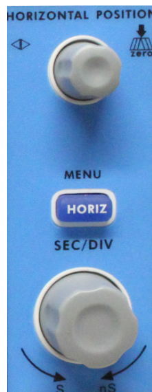
Fig. 11 Horizontal Control Zone
