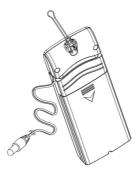
**Note:** Make sure the sensor is mounted vertically and not lying down on a flat surface. This will insure optimum reception. Wireless signals are impacted by distance, interference (other weather stations, wireless phones, wireless routers, TVs and computer monitors), and transmission
