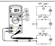
Figure 3-6 Measuring Current
