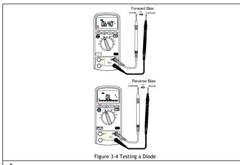
To avoid elecrical shock and/or damage to the instrument, disconnect circuit Power and discharge all high-voltage capacitors before testing diodes.
