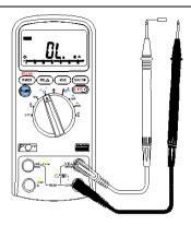
Figure 3-3 Measuring Resistance
