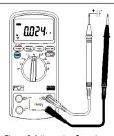
Figure 3-6 Measuring Capacitance
